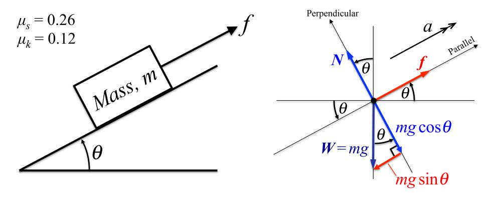
Friction opposes the tendency for the block to slide downhill, so the frictional force must act uphill and parallel to the slope
