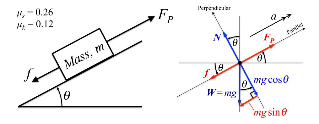
Perpendicular: Parallel:  $N - mg\cos\theta = 0$  $F_P - f - mg\sin\theta = ma$
