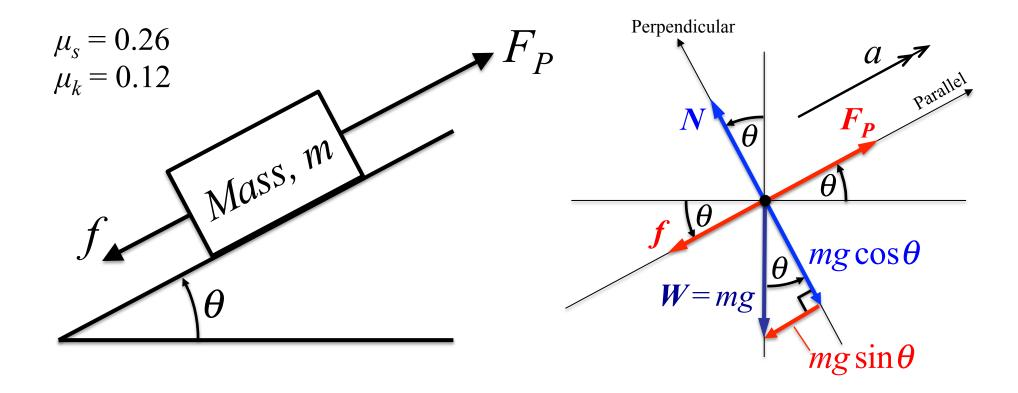
Friction opposes the tendency for the block to slide uphill, so the frictional force must act downhill and parallel to the slope
